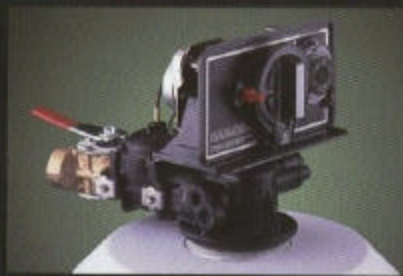
The 5600 with meter measures water usage providing on demand regeneration. This saves water and salt used for regeneration.
